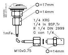
Capillary tube for KP 1A, 5A and 15A
